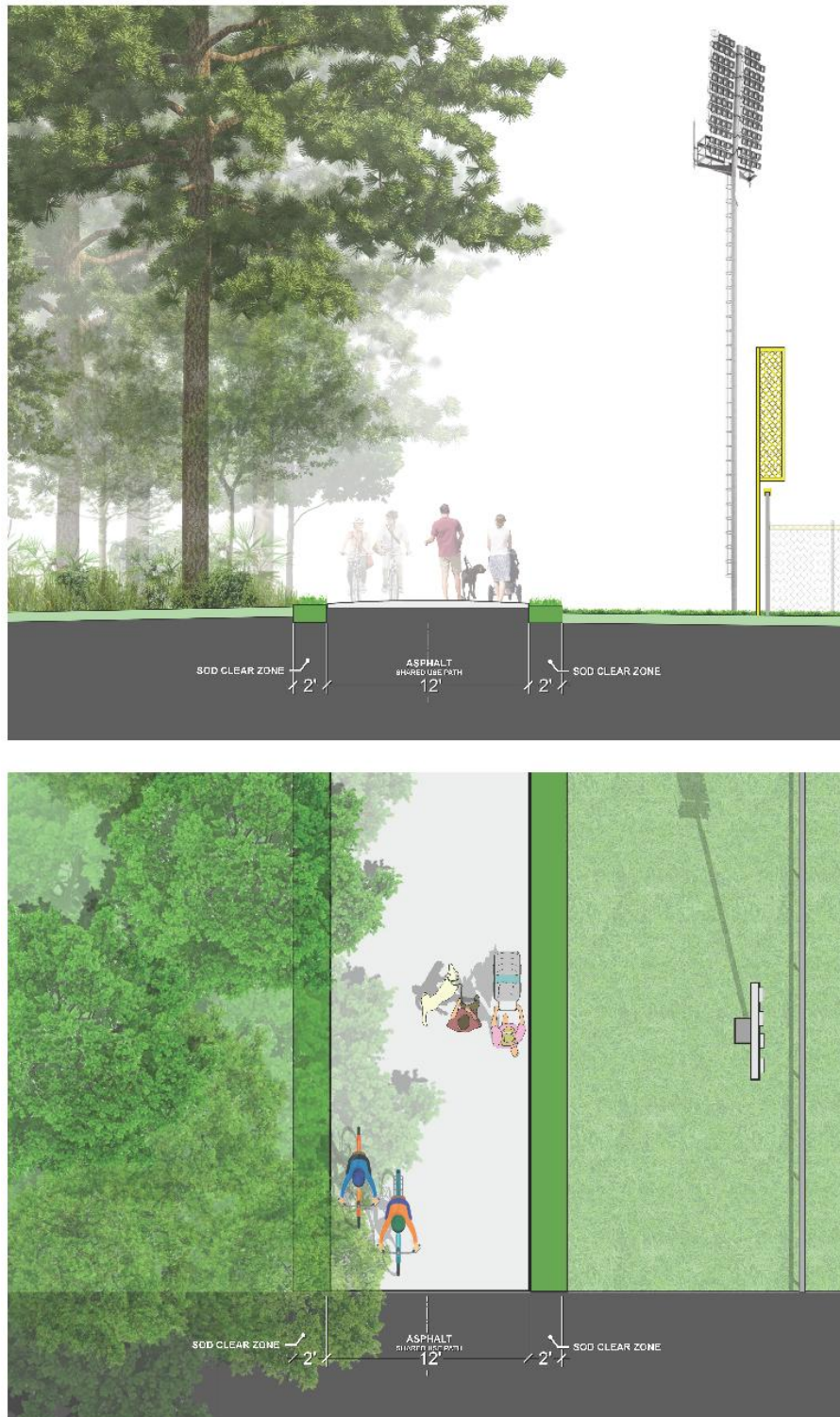
Figure 14: Shared-Use Path Typical Section
