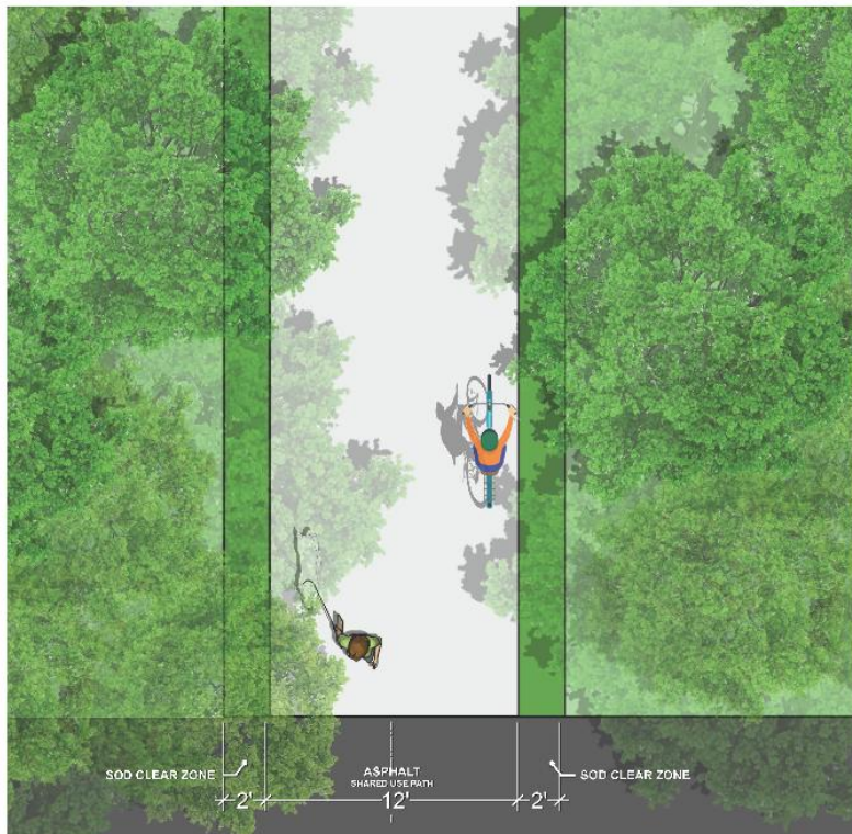
Figure 12: Shared-Use Path Typical Section
