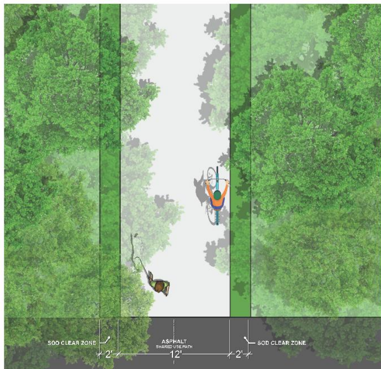
Figure 12: Shared-Use Path Typical Section
