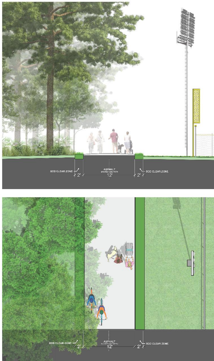
Figure 14: Shared-Use Path Typical Section
