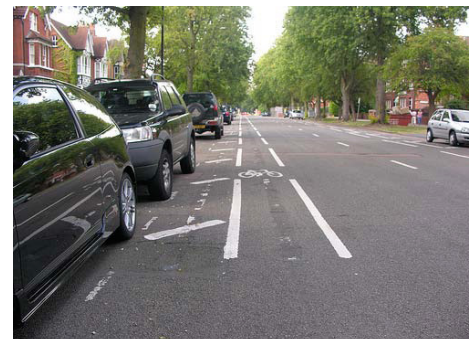
Providing a striped buffer between on-street parking and a bicycle lane is a potential design solution to encourage riding outside the “door zone”.
