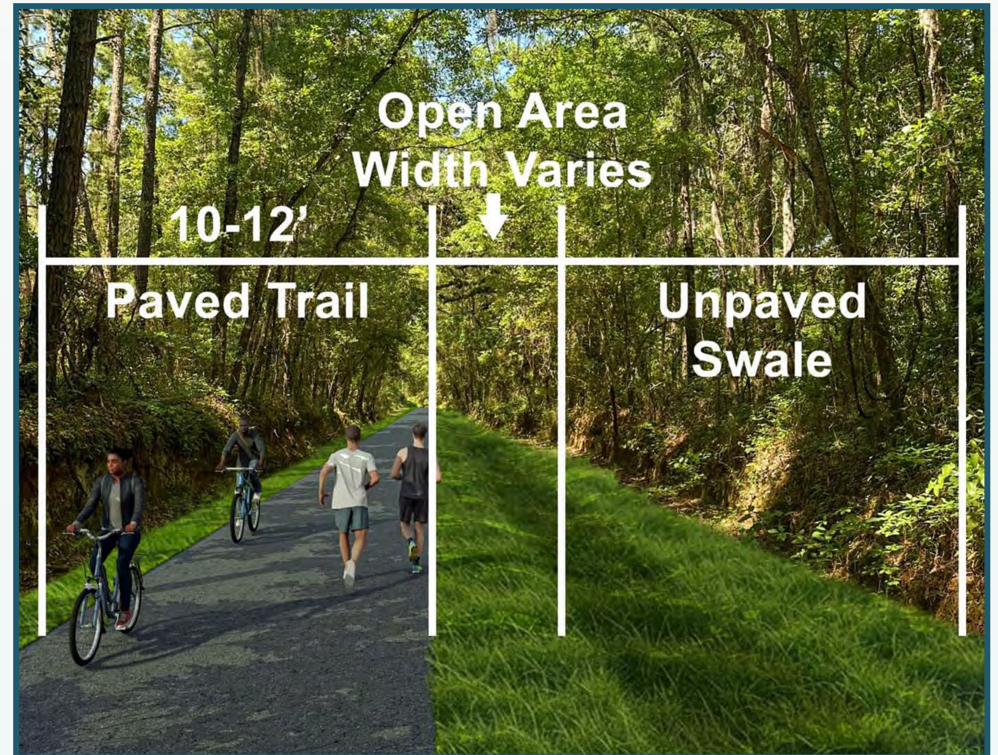
A 10 to 12-foot paved multi-use trail from the eastern trailhead to the western trailhead.
