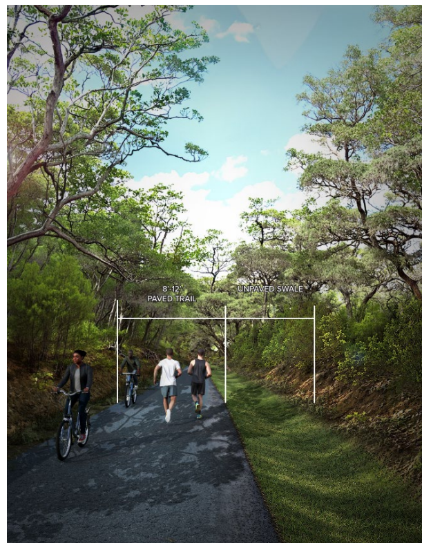
Typical Section – where space is limited
