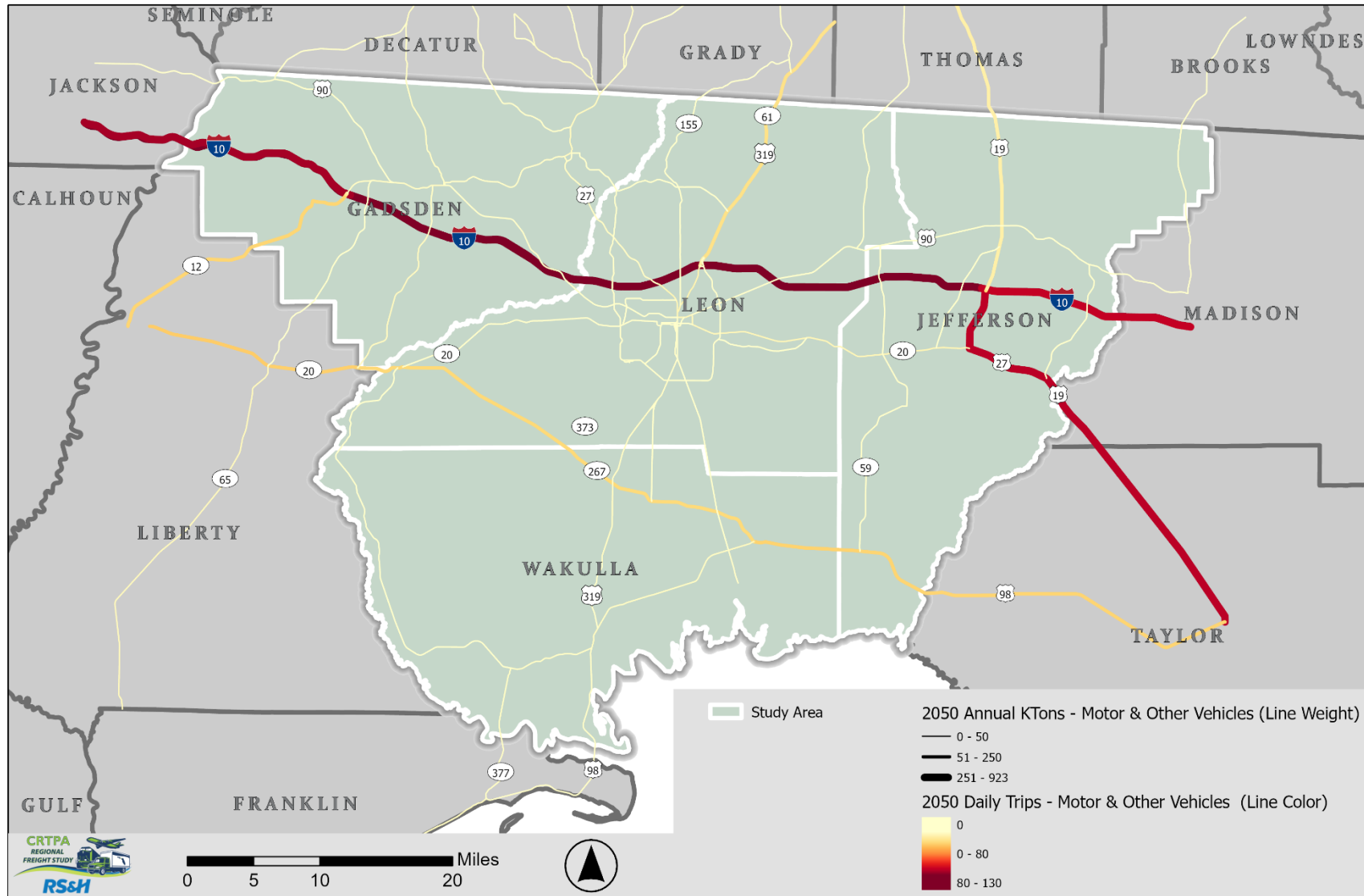
Figure 24: Motor and Other Vehicles Annual Freight Volume (thousand tons) and Daily Trips (2050)
