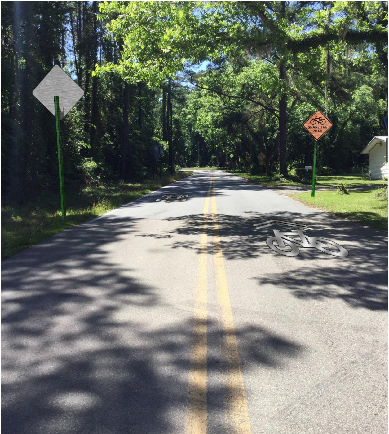
Figure 10: Rendering of shared lane markings on Aucilla Highway
