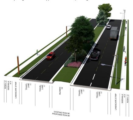
Figure 8 - Springhill Road Typical Section (Orange Avenue to North Lake Bradford Road)
