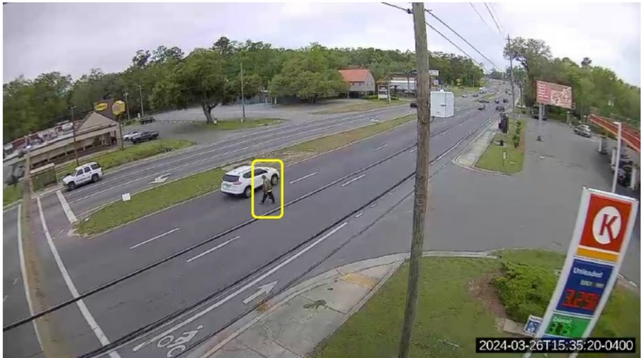
Figure 4: Pedestrian starts crossing westbound near the Gas Station driveway and passes near an incoming vehicle entering US Hwy 27 from the east leg of Sharer Rd. It represents a near-miss case where the driver had to evade the pedestrian. (Date 03/26/2024 at 3:35 PM)
